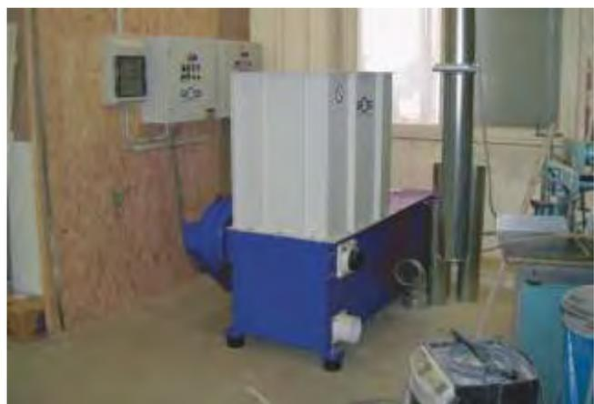
GAZ 62 shredder connected to an air suction system
